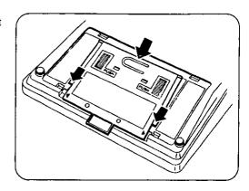
2 While pushing on the areas marked "PUSH", insert the edges of the holder under the slide rails and then slide in the direction of arrow .
